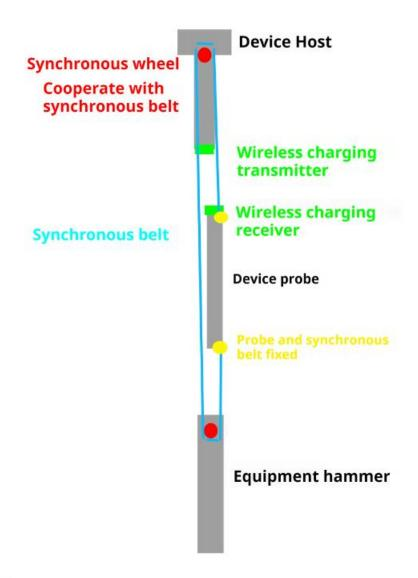
Each set of equipment is composed of three parts, the main machine, the probe, the weight, and the synchronization belt is connected; The main engine provides power, the probe collects data, and the synchronous belt is assisted by the vertical force of the weight; After the probe completes the collection, the data is
